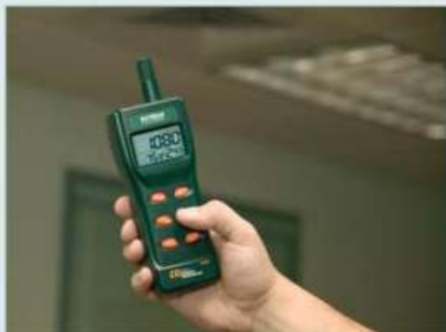
Measure CO 2 level in office buildings to check the air quality of conference rooms insuring proper ventilation.
